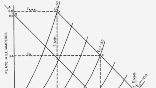
Example: Determine the undistorted power output of a 3-electrode tube at a plate voltage of 250 volts, a plate current of 34 milliamperes, a negative grid voltage of 50 volts and a plate load of 3900 ohms; given the plate characteristic curves as shown.
