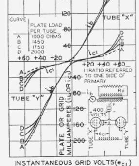
that is, the primary input voltage is higher than the secondary voltage supplied to the grids of the power output tubes. Depending upon conditions, the ratio of the primary of the interstage transformer to one-half of its secondary may range between 1.5 to 1 and 5.5 to 1. The transformer step-down ratio is dependent on the following factors: (1) Type of driver tube, (2) Type of power tube, (3) Load on power tube, (4) Permissible distortion, and (5) Transformer efficiency (peak power).
