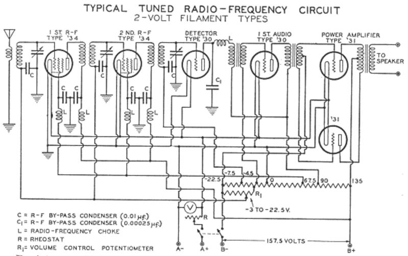
Resistance Strip = The values of the respective resistors in this strip should be chosen to give the indicated voltages at the various taps, as measured with a high resistance voltmeter. The total resistance in the strip should have a value such that the bleeder current will be approximately 8 milliamperes.
