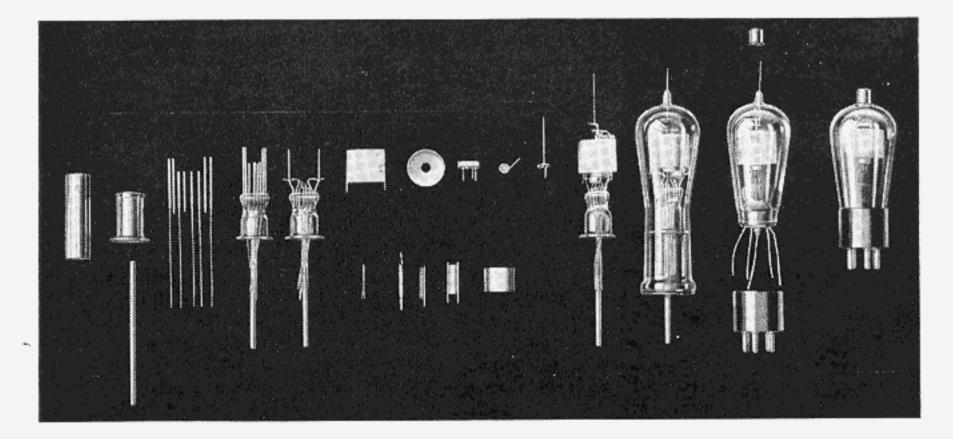
Parts Assembly of the '24-A
