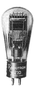
Grid bias for the type '10 may be obtained from a C-supply or by means of the voltage drop in a resistor connected in the negative plate return lead. The latter method is known as the self-biasing method, since the plate current determines the drop. It is not, however, generally applicable to battery-operated receivers.
