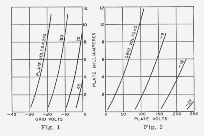
Dynamic characteristics include amplification factor, plate resistance, and mutual conductance, and may be shown in curve form for variations in tube operating conditions.
