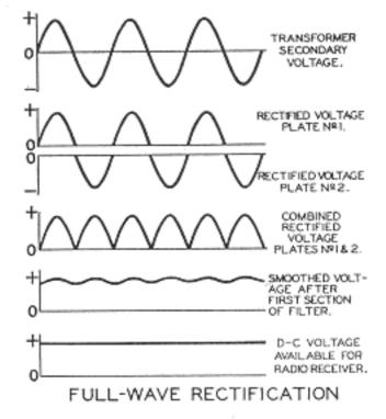
tube, current may be obtained on both halves of the a-c cycle. The '80 is an example of this type and is called a full-wave rectifier.
