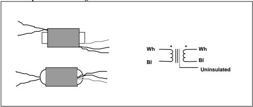
Static resistance of primary $260 \Omega$ Static resistance of secondary $205 \Omega$
