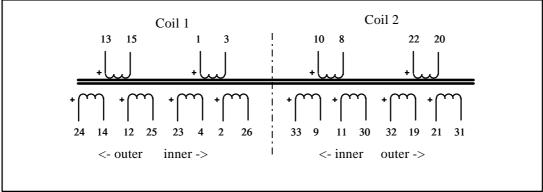
Static resistance of each primary (avarage): $0.80 \Omega$ Static resistance of each secondary (avarage): $0.40 \Omega$ Max voltage per primary winding, at 50 Hz:40 voltsMax voltage per secondary winding, at 50 Hz:20 volts
