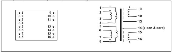
Spacing between pins:2.54 mm (0.1")Spacing between rows of pins:22.86 mm (0.9")Weight:30 gRec. PCB hole diameter:1.5 mmStatic resistance of each primary (average): $22 \Omega$ Static resistance of each secondary (average): $45 \Omega$ Self resonace point:> 500 kHz
