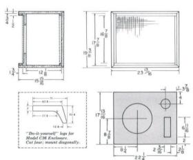
These minimum-volume reflex enclosures will accommodate a variety of loudspeaker components. Model C36 is an upright enclosure which uses the diagonal legs shown here. Model C38 is a lowboy version of the same enclosure which uses tapered wooden legs. Two of these reflex units with appropriate loudspeakers installed make an excellent space-saving stereo speaker installation.
